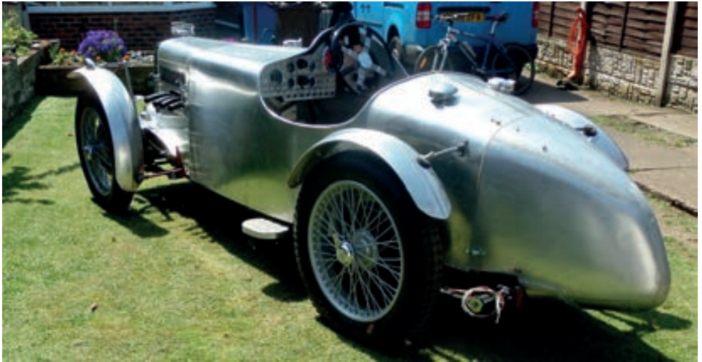
Top: The body temporarily fitted to the chassis. Dummy exhaust manifold visible at front.
